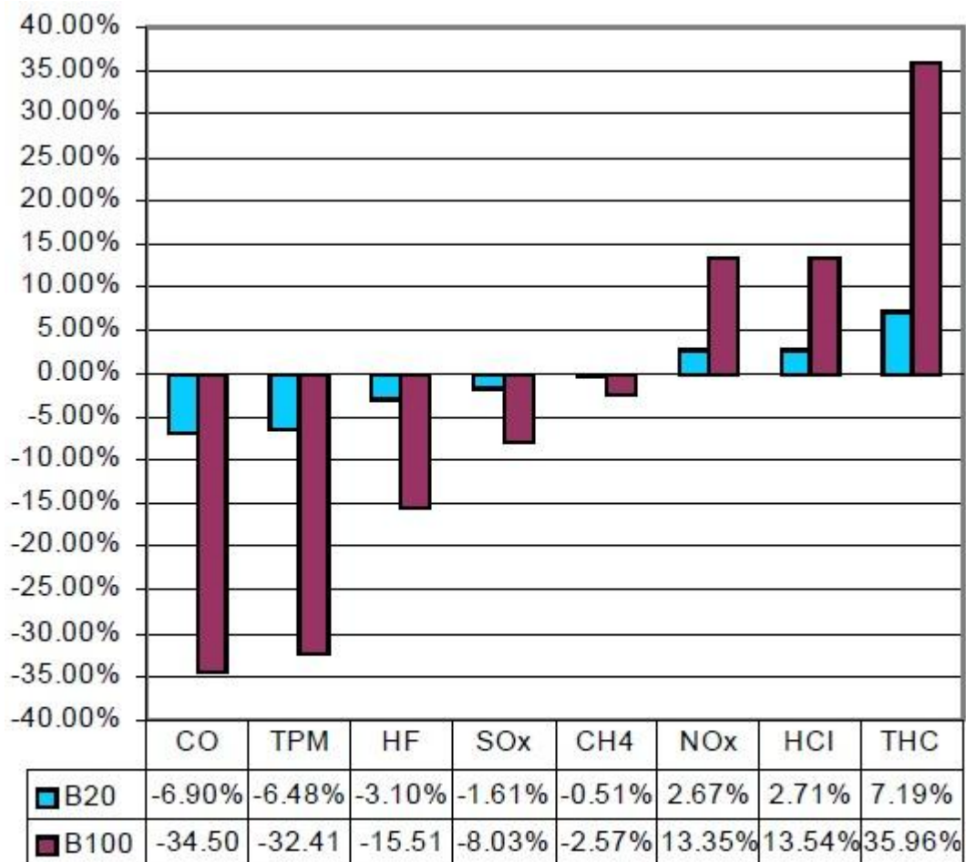
Figure 3. Life Cycle Air Emissions for B100 and B20 Compared to Petroleum Diesel
